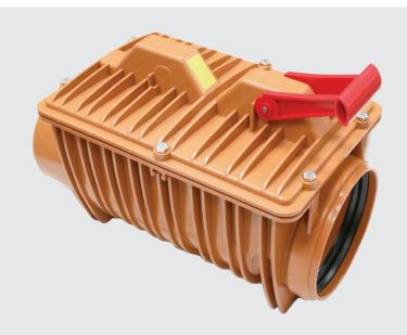
Backwater Valves are installed in-line with the drainage system, allowing sewer or surface water materials to travel freely in the direction of flow but blocks backflow of those materials in the opposite direction in instances, such as, flooding.
